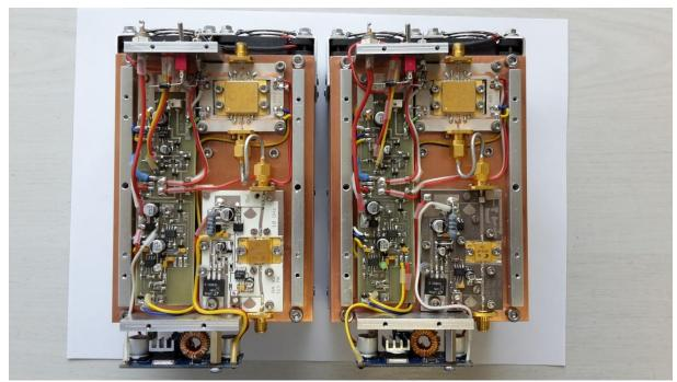
Figure 1. Two 10 GHz power amplifiers with TGA2312FL
