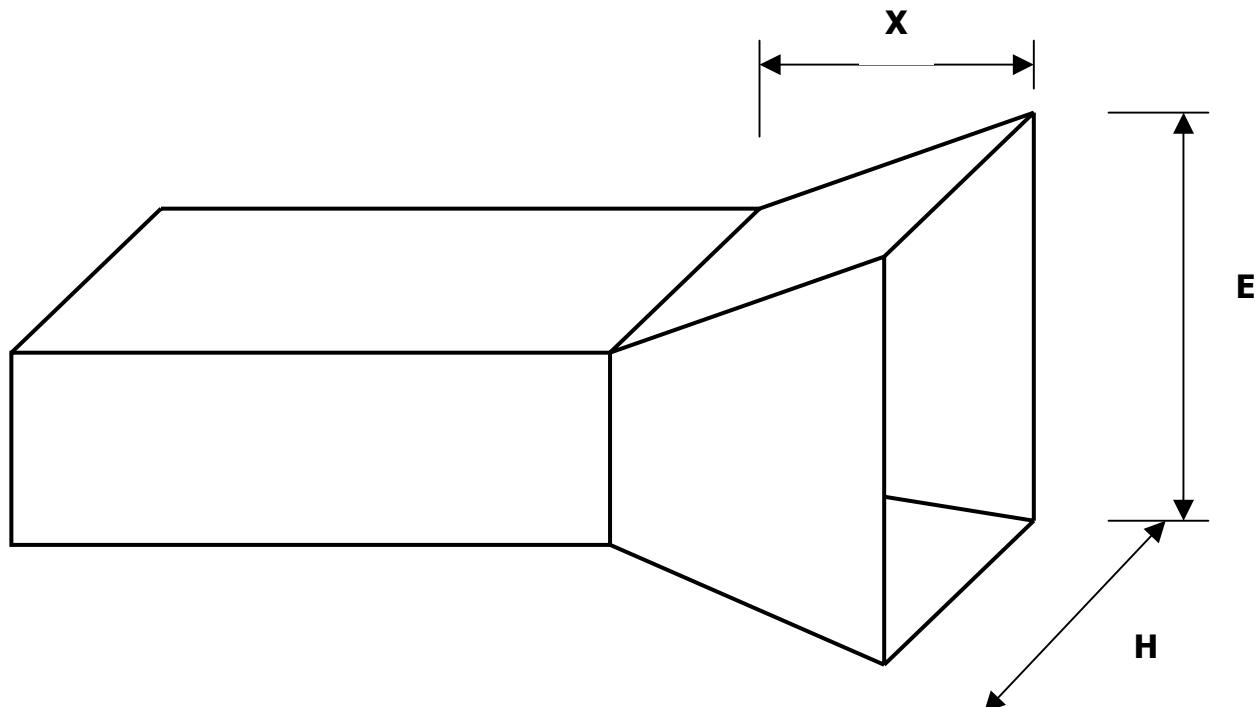
Practical solution 1296 MHz show, that for f/D 0,5 ratio is optimum size 180 x 180 mm on the flare aperture and f/D ratio 0,45 is optimum size 157 x 157 mm.
