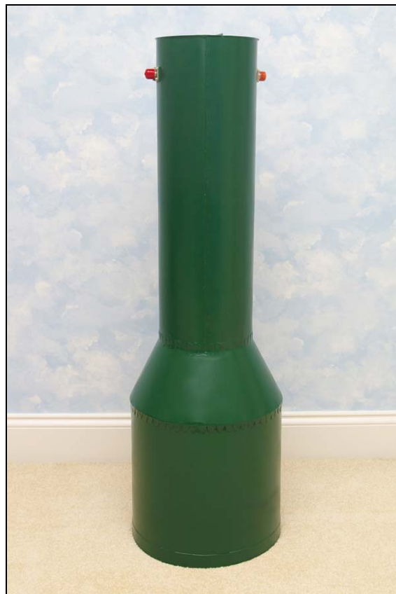
Fig. 19 – View of the feedhorn after tuning and painting
