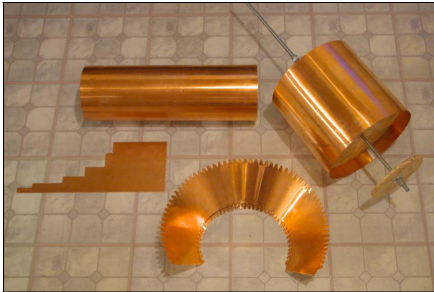
Fig. 17 – Various feedhorn pieces during construction
