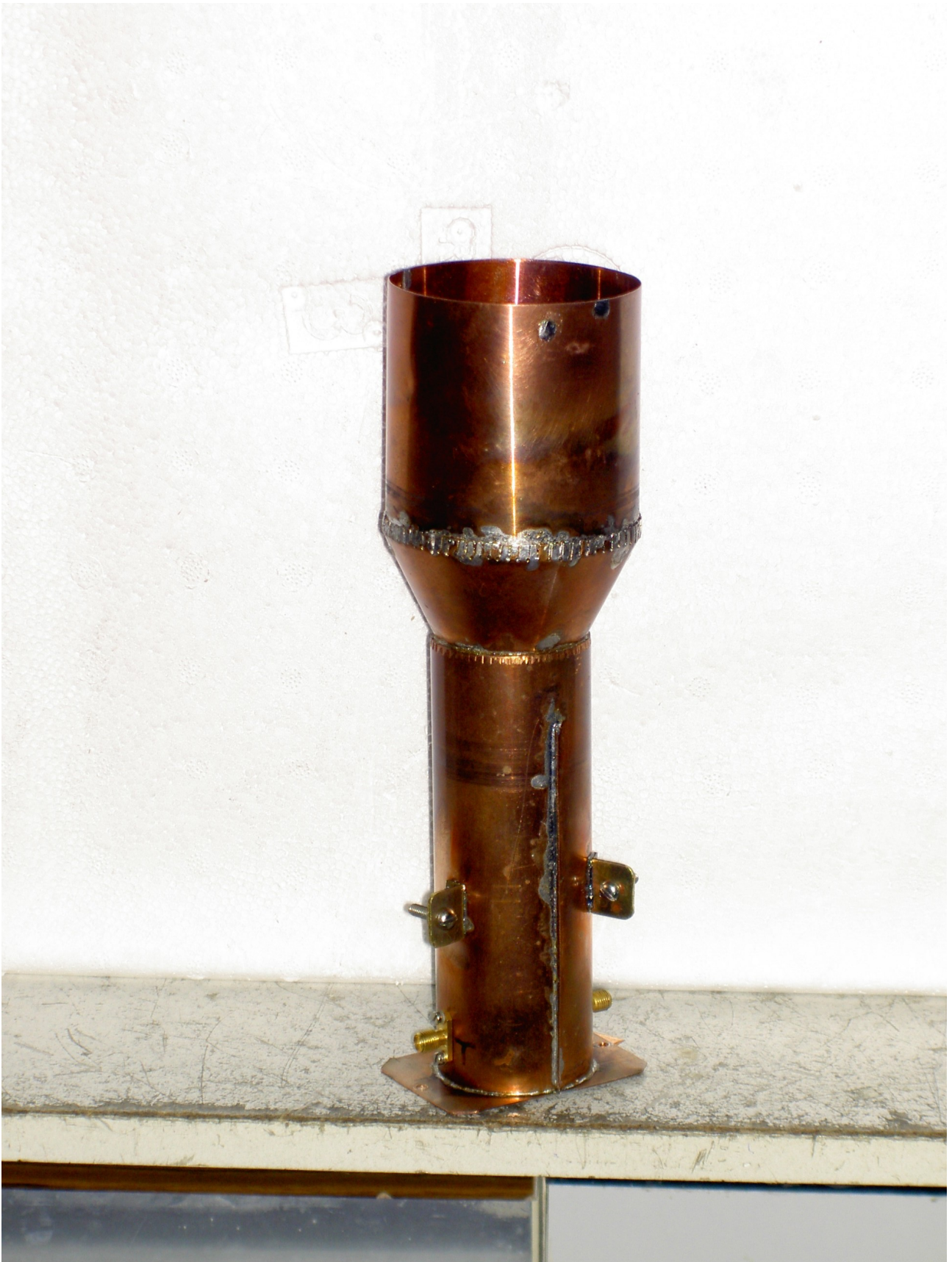
The Completed 6cm Dual Mode Horn
