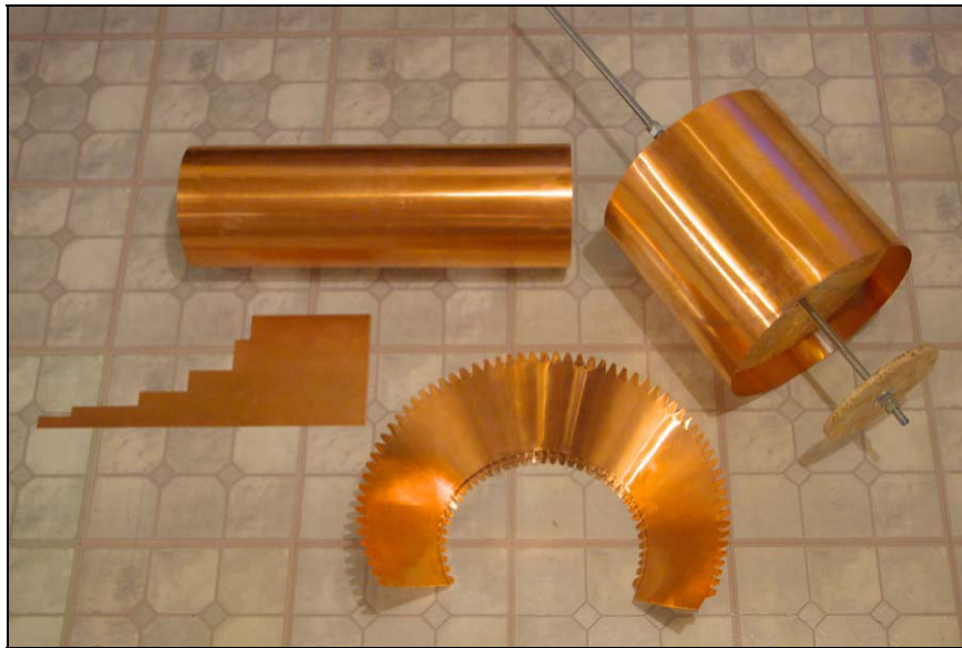
Fig. 17 – Various feedhorn pieces during construction
