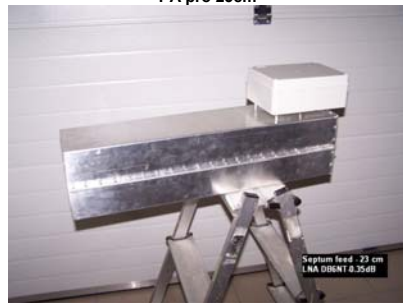
Septum feed - 23 cm LNA 035dB @ 3.5dB
